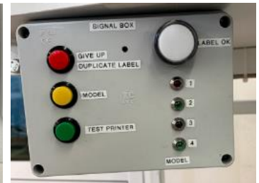
Figure 2: TCIS control and signal box
